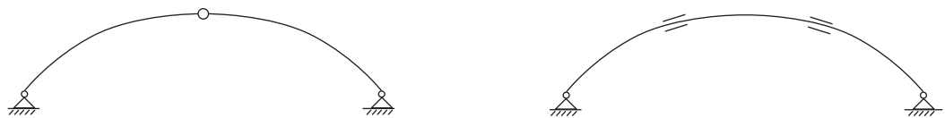
Figure 3.43 Suitable placing of joints in arch structures. Left: Hinge, Right: Rigid joints.
