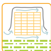
Ventilation under presenning
